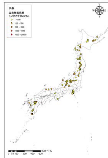
Figure 11 Resource distribution chart for hot spring power generation where Rankine cycle is assumed
